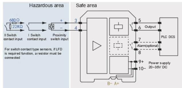
Note: The power supply of the power rail is an optional function. Users need to specify the power supply mode when ordering. Please refer to attachment on page 89.
