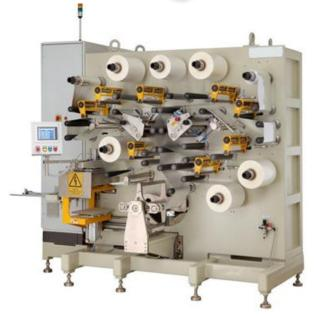
**Application:** monitoring a jockey roller in electronic components manufacturing. **Need:** different materials have to be assembled with high precision. The jockey rollers are used to keep the different foils at the right tension.
